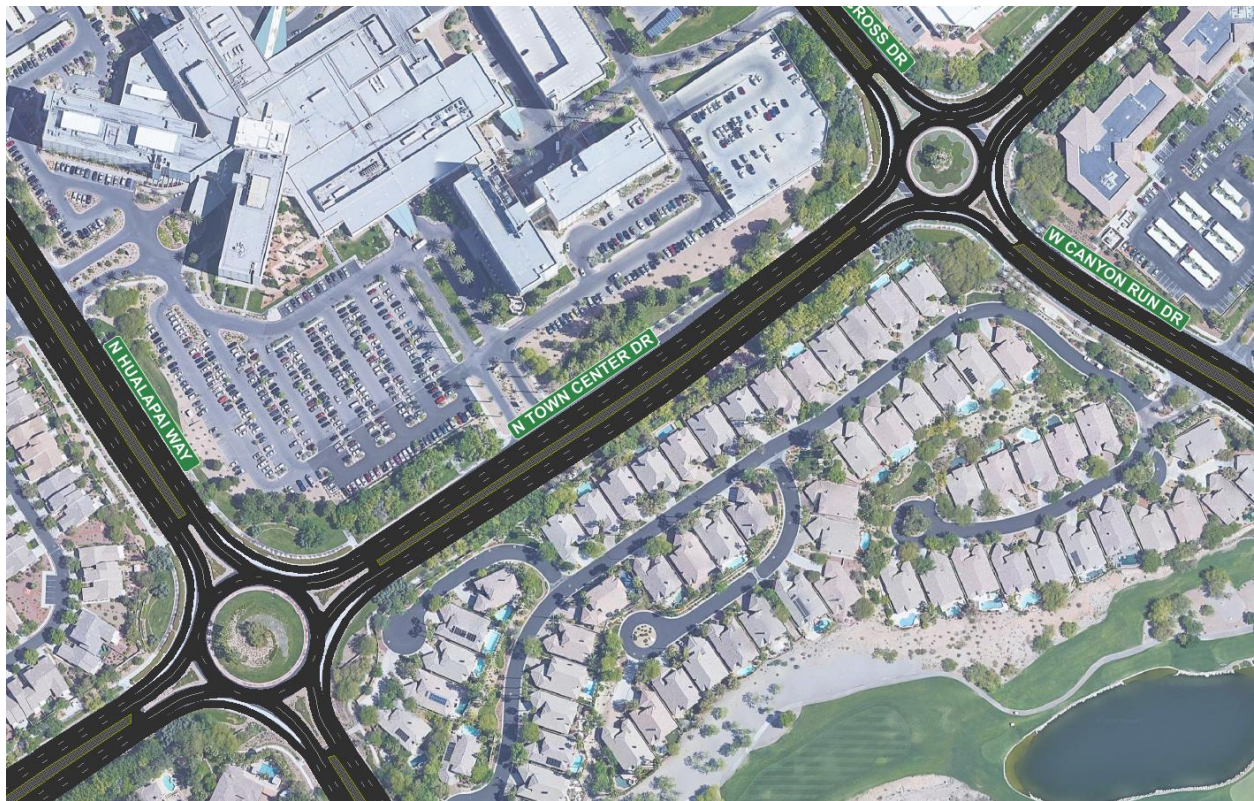
Figure 2-2. A pair of roundabouts along N. Town Center Drive
